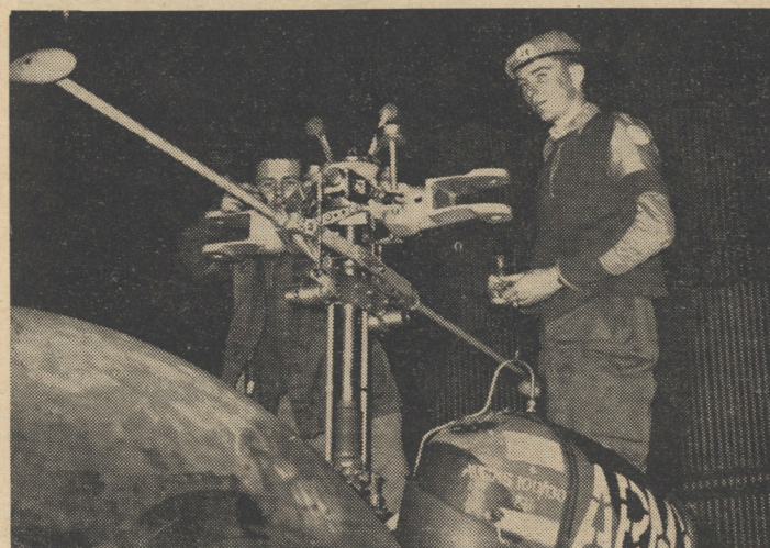
Cpl Tony Duffy (left) and Lcpl Andrew Baird servicing and re-assembling the main rotor assembly of a Sioux.
